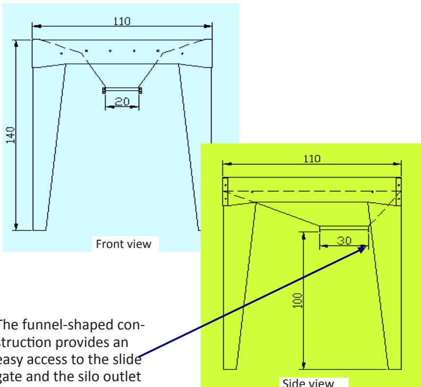
The funnel-shaped construction provides an easy access to the slide gate and the silo outlet passes the front legs
